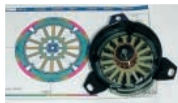
Figure 2: ECF motor with bonded Neo arcs and armature in the process of reworking.
