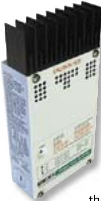
A wind-electric charge controller's primary function is to protect your battery bank from overcharging. It does this by monitoring the battery bank—when the bank is fully charged, the controller sends energy from the battery bank to a dump (diversion) load.
