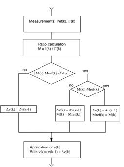
Fig. 6. Optimal control algorithm
