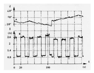
Fig. 5. I(t) and v(t) (variable load)
