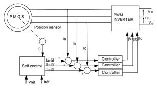
Fig. 2. Basic Voltage Source Converter structure
