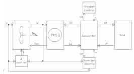
Fig. 1. Wind Turbine using PMSG
