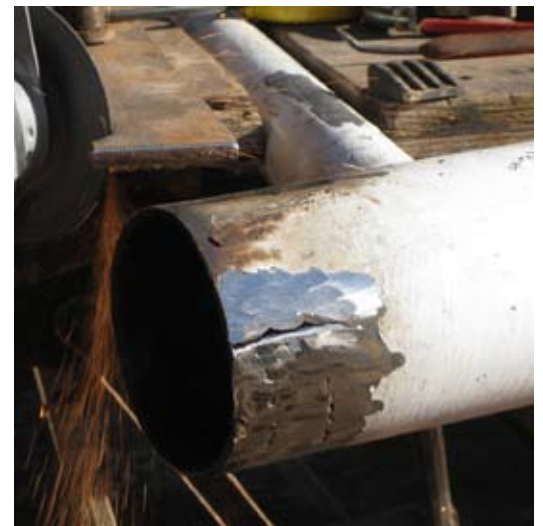
Fig. 44: Crack tail vane
