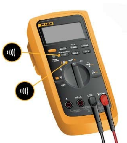
Fig. 53: Multimeter on continuity position
