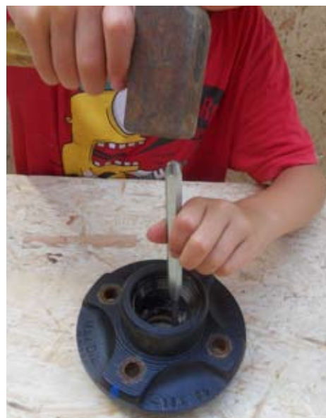
Fig. 38: Take out the outer shell
