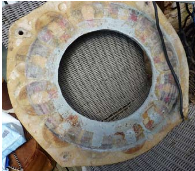
Fig. 31: Friction on the stator
