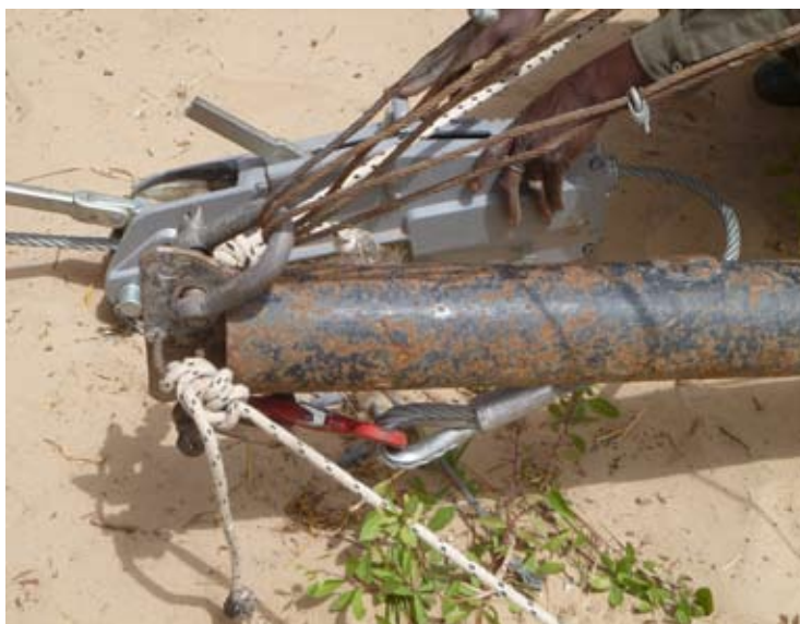
Fig. 11: Extremity of the gin pole with the rope hoist
