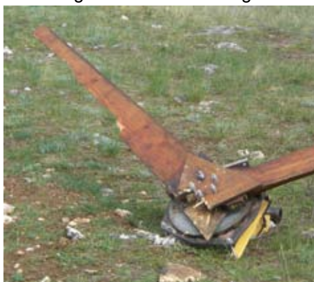
Fig. 63: Loss of balancing weight
