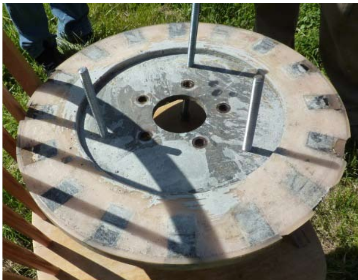
Fig. 30: Front rotor with the 3 jacking screws
