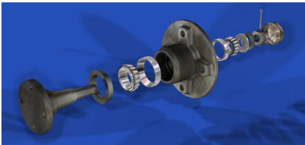
Fig. 36: Exploded view of a whole bearing
