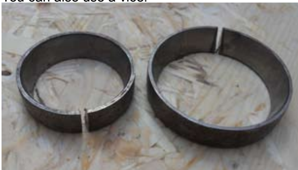
Fig. 39: Cut the shell with an angle grinder
