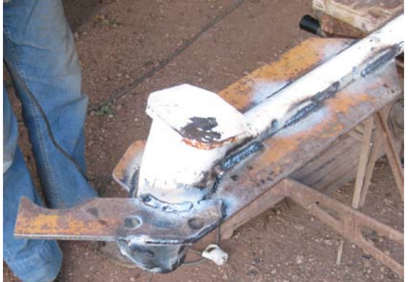
Fig. 43: Reinforced tail vane
