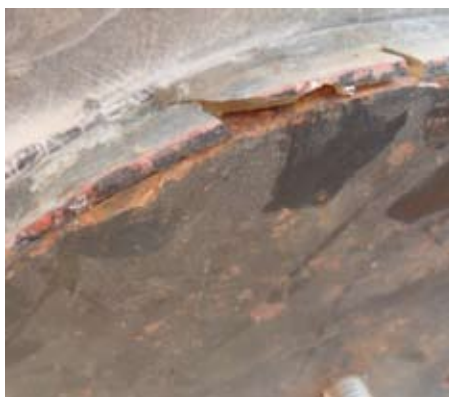
Fig. 33: Cracks in resin in the rotor edge
