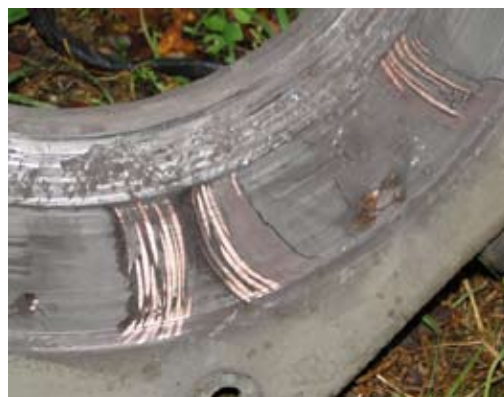
Fig. 34: Stator that needs to be changed
