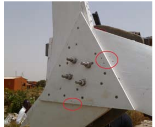
Fig. 18: Marks on blades and triangle
