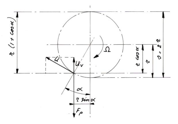
fig. 3 Pump rod directly driven by a crank on the rotor shaft
