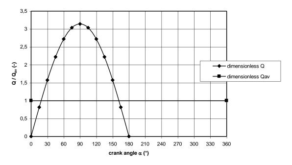
fig. 1 Dimensionless torque Q /  $Q_{av}$  and dimensionless average torque  $Q_{av}$  /  $Q_{av}$  as a function of the crank angle  $\alpha$
