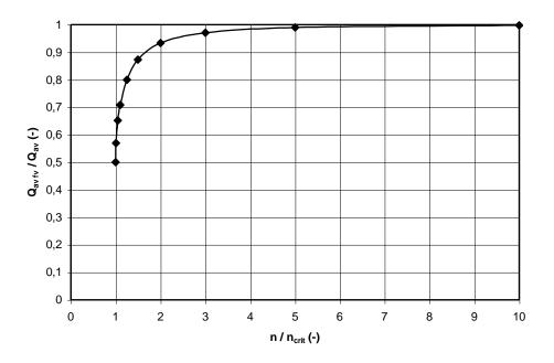
fig. 4 Values of  $Q_{av fv} / Q_{av}$  as a function of  $n / n_{crit}$
