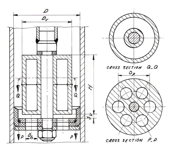
fig. 2 Cross section of piston and floating valve
