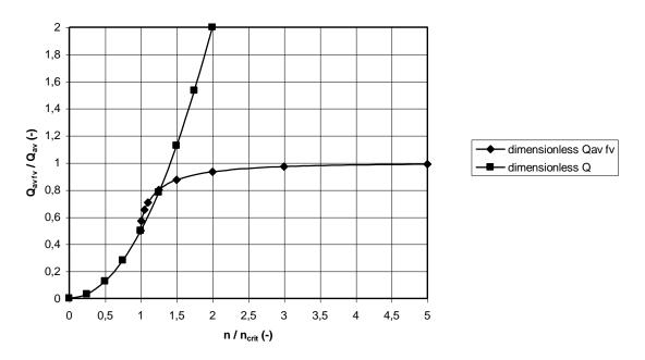
fig. 5 Values of  $Q_{av fv}$  /  $Q_{av}$  and optimum rotor torque Q /  $Q_{av}$  as a function of n /  $n_{crit}$
