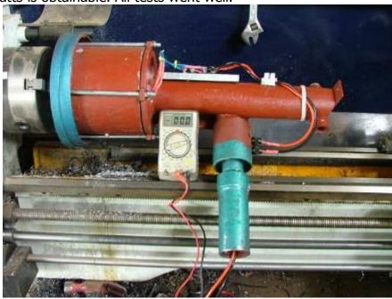
EcoInnovation added a 3-phase rectifier and secured the cable from chaffing. Note the two brush holders on the bottom right of the picture.
