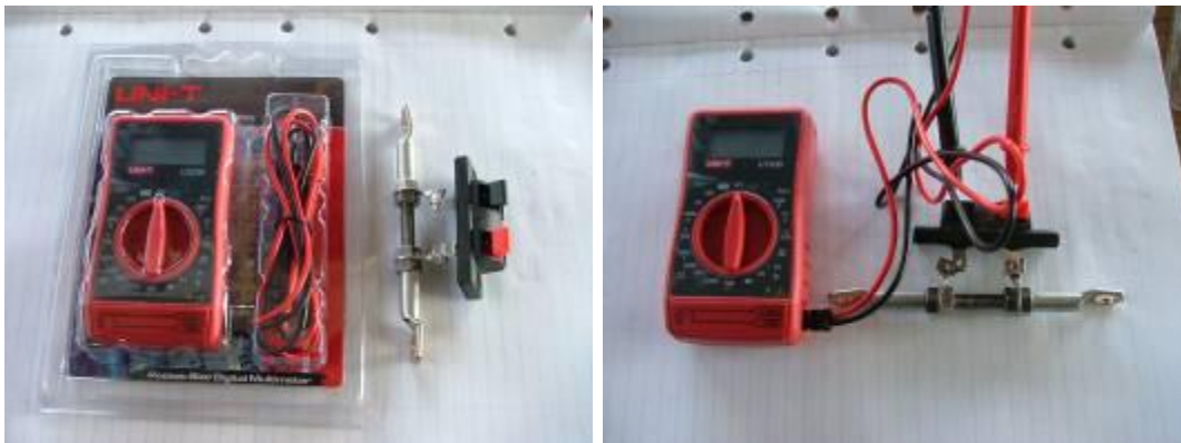
Uni-T multi-meter and shunt
