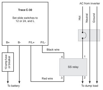
control rated from 90 to 280 VAC and contacts rated at 25 A from 24 to 330 VAC. That's plenty of range and headroom. See the schematic for details.
