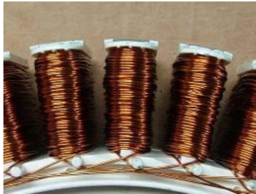
Resistance of each phase = 15.2 ohms
