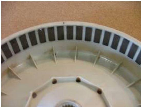
Type 1 rotor (old design)
