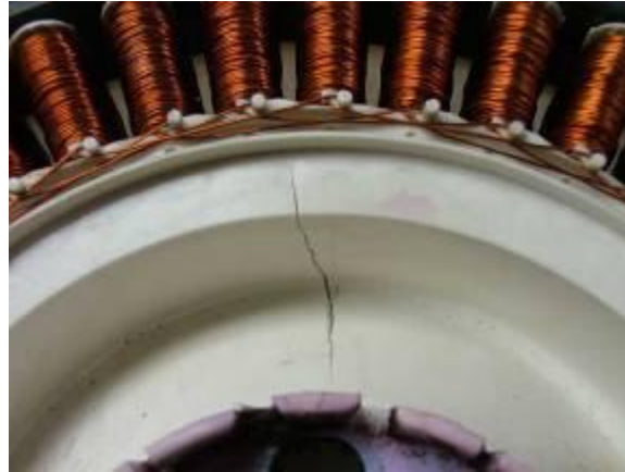
Typical crack on an inventors kit stator
